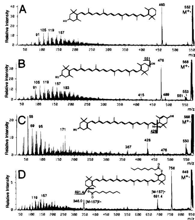
**Figure 3.** FAB MS-MS mass spectra (linked scanning at constant B/E with CAD) of the alcohol- and ester-containing xanthophylls (A)  $\beta$ -cryptoxanthin, (B) zeaxanthin, (C) lutein, and (D) isozeaxanthin bis(pelargonate).
