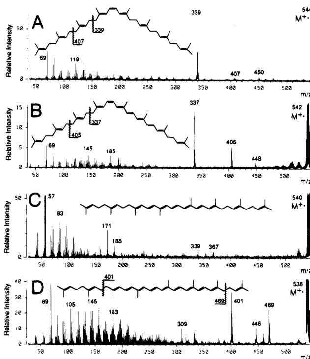
**Figure 1.** Positive ion MS-MS spectra obtained using FAB ionization, collisionally activated dissociation (CAD) of molecular ions, and linked scanning at constant B/E of the fragment ions for the lycopene metabolic precursors (A) phytoene, (B) phytofluene, (C)  $\zeta$ -carotene, and (D) neurosporene.
