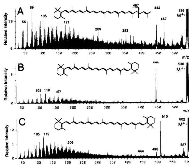
**Figure 2.** Positive ion FAB MS-MS spectra (linked scanning at constant B/E with CAD) of the carotenes (A)  $\gamma$ -carotene, (B)  $\beta$ -carotene, and (C) nonaprene.
