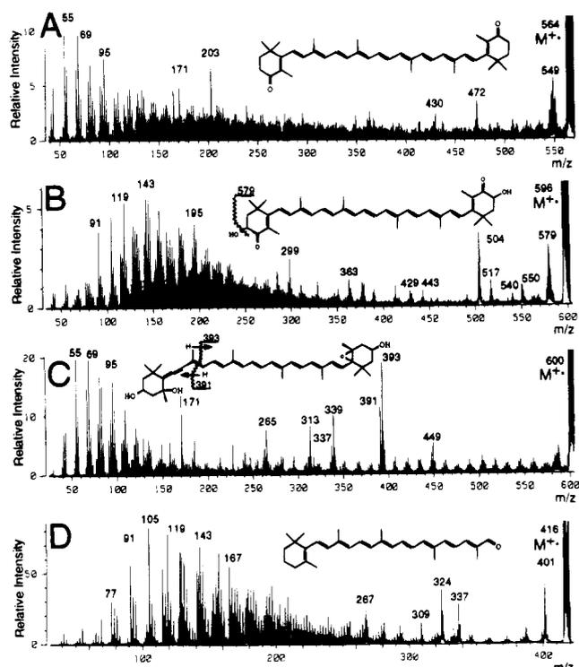
**Figure 4.** FAB MS-MS mass spectra (linked scanning at constant B/E with CAD) of the xanthophylls (A) canthaxanthin, (B) astaxanthin, (C) neoxanthin, and (D)  $\beta$ -apo-8'-carotenal.
